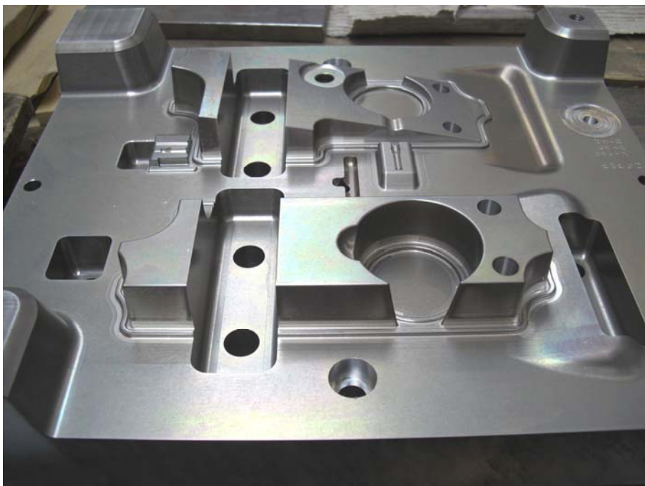
Injection-moulding mould made from aluminium by sauer product (photo: sauer product)
