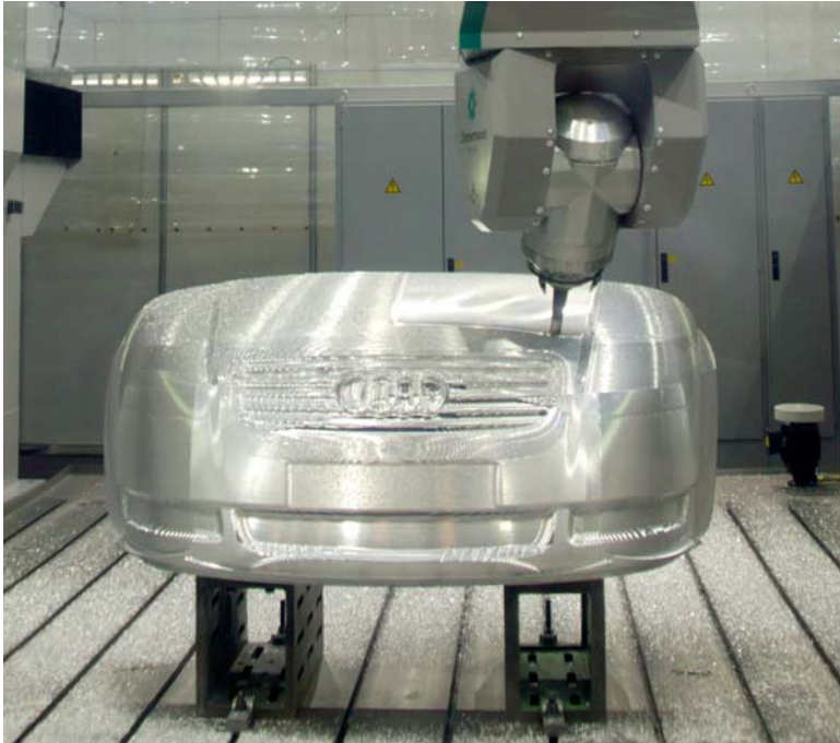
Aluminium's good machinability makes short processing times possible even with large-format parts (photo: Klaus Vollrath)
