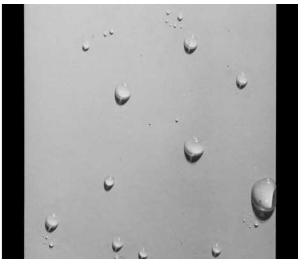
Highly water-repellent surface with little wetting following use of a Type I b or Type II cleaning agent (Fig. 2.1)
